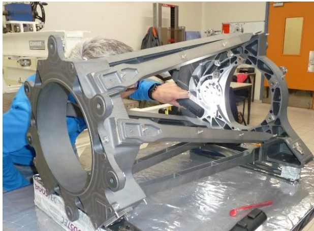
Fig. 9. STM main structure assembly at DRB
